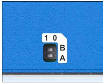
Figure 2.7: Ground reference switches
